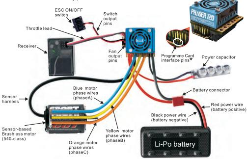
\* Programming card interface pins allows you to connect the program card directly to your ESC for easy programming.
